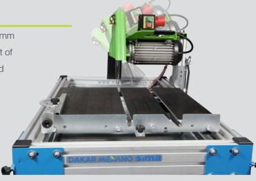
90% of the machine is manufactured of stainless materials. The rest is painted with a anti-corrosion epoxy-polyester coating.
