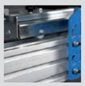
60% of the machine is manufactured of stainless materials. The rest is painted with a anti-corrosion epoxy-polyester coating.
