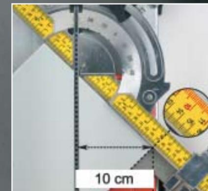
Goniometric square in "45°" position for a direct reading of the measurement for diagonal cuts.
